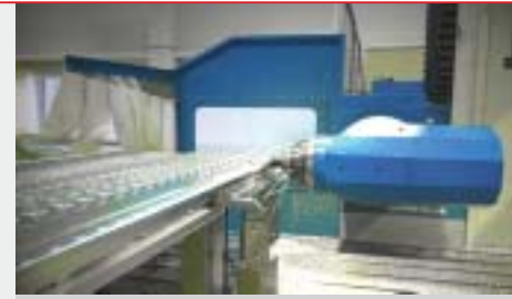
5-axis milling machine processing structure components for aviation
